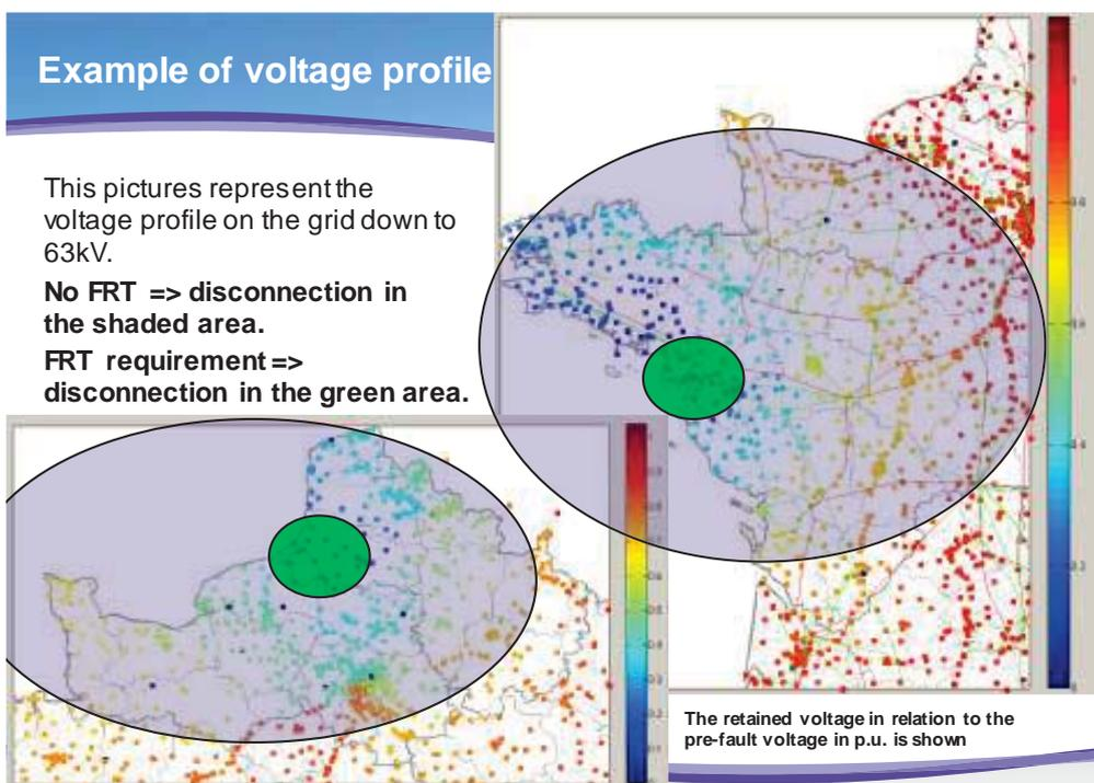
The retained voltage in relation to the pre-fault voltage in p.u. is shown
