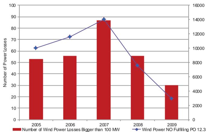
Number of losses of more than 100 MW of wind power per year (red columns) versus evolution of wind power without FRT (blue line).
