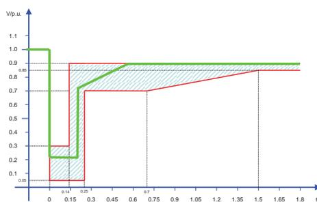
➤ Profile determined by the standard (Green Line) is fully compliant with the RfG code.
